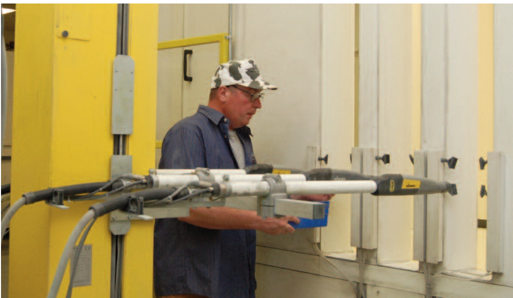
Long-stroke vertical reciprocators with horizontally mounted spray guns dramatically improved transfer efficiency, lowering material use.
